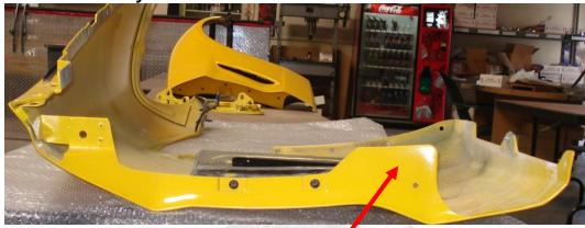
Drill new hole for support bracket. use M6x1 bolt.
