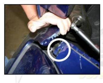
Pull upward on front bumper cover as shown and remove screw with T15 Torx wrench. Continue removing the rest of the T15 screws front the top of the fender.
