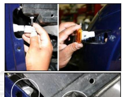
Look inside inner fender and above where the turn signal was, unscrew three bolts.
