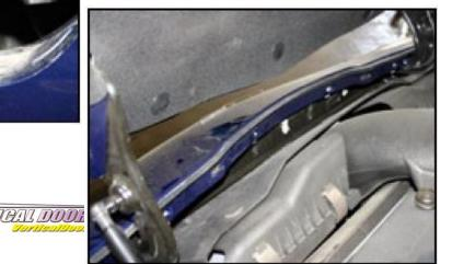
Using 7mm socket, remove (4) screws from front bumper cover underneath hood area.
