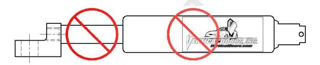
WARNING! THE USE OF ANY TYPE PLYERS, PAINT OR FOREING MATERIALS ON THE SHOCK'S BODY OR SHAFT WILL VOID THE WARRANTY.
