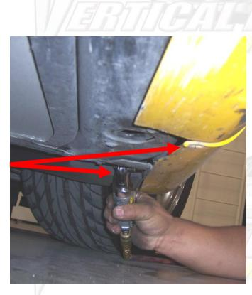
Remove (2) 7mm bolts from the bottom of the fender.
